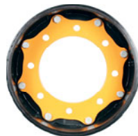
Hub Adapter MSPN 47139 CAI 419992 12 mm thick 1015 carbon steel / reversible 8.75" (222.3 mm) center dia. 8 x 10.91" bolt pattern 0.79" (20 mm) bolt holes, no taper Fits front of Case backhoe loader machines
