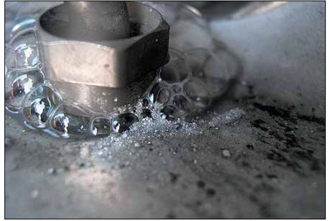
Corrosion-Related Leak at the Base of the Wheel
