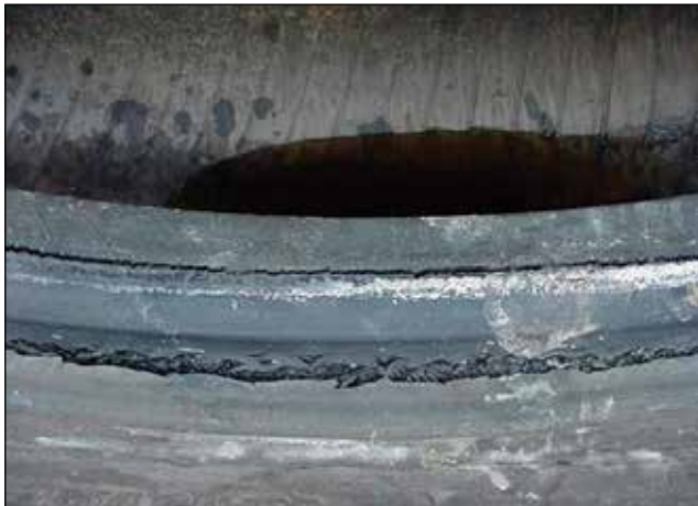
2nd Stage – Bead Splitting from Heat
