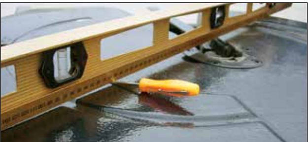
Distortion of the 5th Wheel
