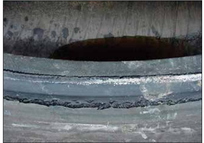
2nd Stage – Bead Splitting from Heat
