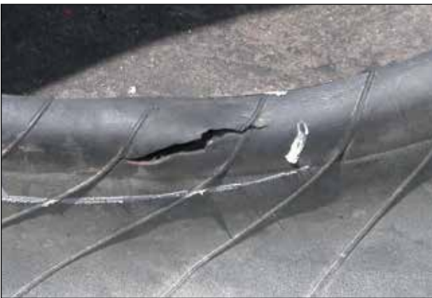
Bead Damage Caused by Mounting/Dismounting
