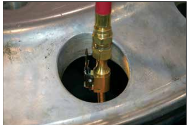
12 Use a clip-on chuck and allows for a sufficient length of the hose to extends outside the safety cage.
