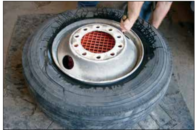
10 With assembly horizontal, inflate to no more than 5 psi to seat the beads.
