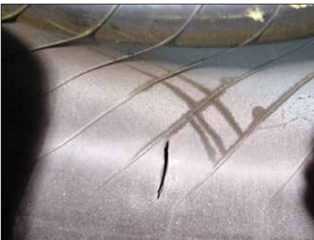
EFFECT: Inner Liner Split CAUSE: Sidewall Impact
