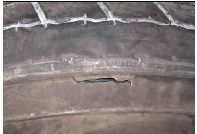
Sidewall Rupture Shock
