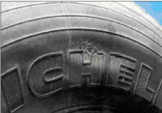
EFFECT: Small Bulge CAUSE: Impact with a Curb, Pothole, Road Debris, etc.
