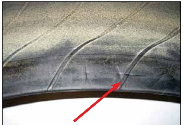
Severe inner liner damage from use of hammer.
