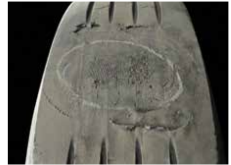
Brake Skid Damage
