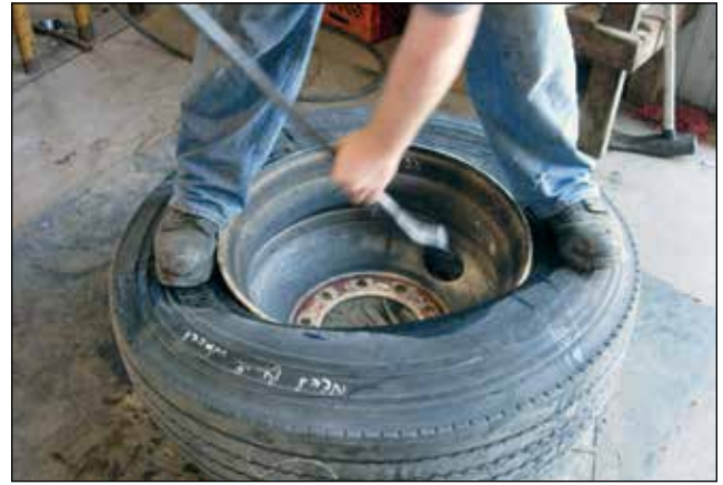
8 Mount second bead using same method.
