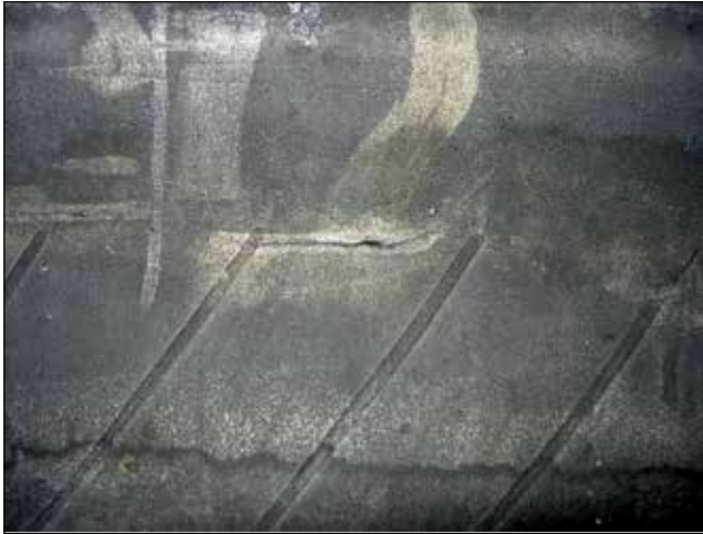
EFFECT: Inner Liner Cut CAUSE: Shipping or Mounting Damage
