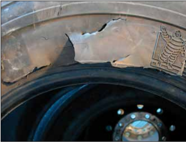
EFFECT: External Rubber Damage CAUSE: Severe Impact
