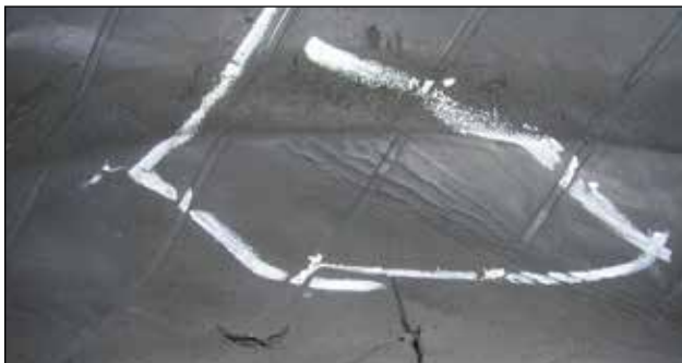
Inner Liner Marbling/creasing
