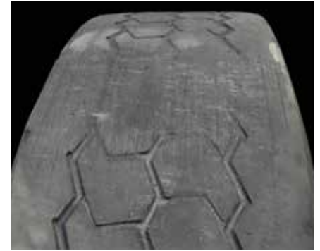
Brake Skid Damage
