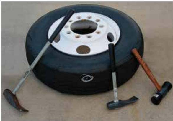
Only use a duck bill hammer as a wedge with a rubber mallet.
