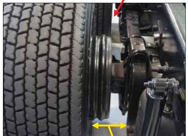
Correct Lateral Clearance
