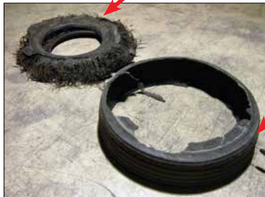
EFFECT: Run Flat CAUSE: Crown Perforation/Penetration
