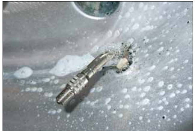
Corrosion-Related Leak at the Base of the Wheel
