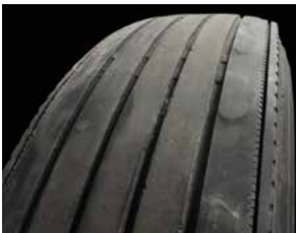
Depression Wear (Shoulder)
