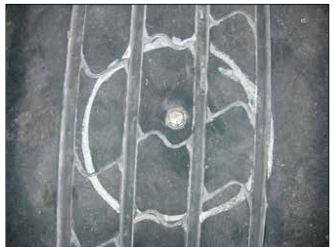
EFFECT: Object that Penetrates into the Tire and Through the Inner Liner CAUSE: Nail, Bolt, Screw, etc.
