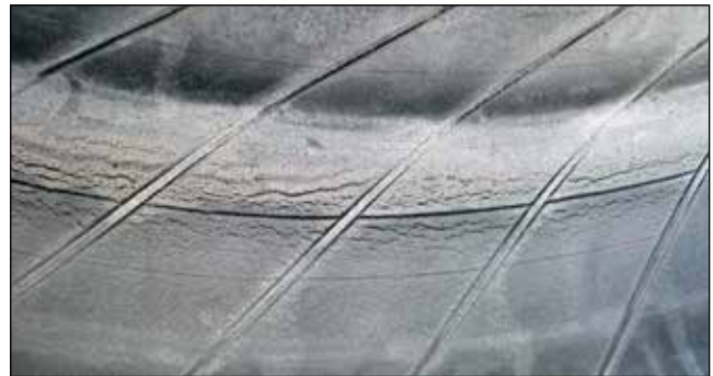
EFFECT: Inner Liner Cracking CAUSE: Underinflation
