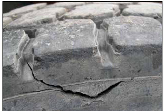
Sidewall Area Damage
