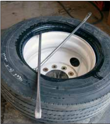
7 Completely unseat the first bead.
