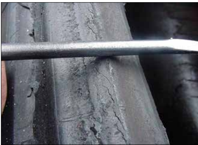
1st Stage – Turning of the Bead
