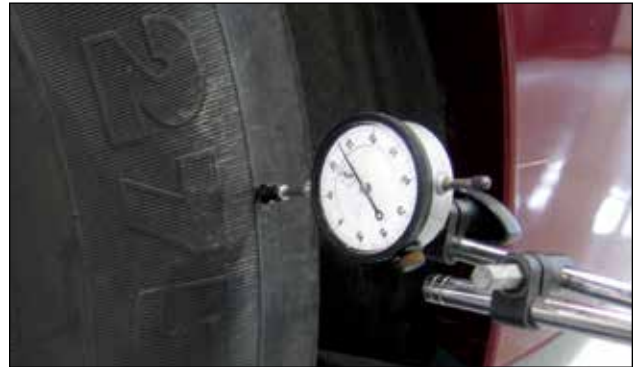
Measuring Lateral Runout on Outside Shoulder
