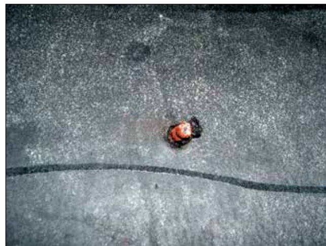
EFFECT: Premature Failure of Repair CAUSE: Object that Penetrates into the Tire and Through the Inner Liner
