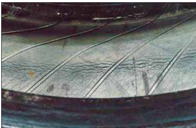
Potential Zipper Rupture
