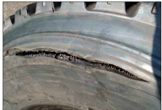
Zipper Resulting from Run Flat Condition
