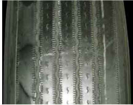
Depression Wear (Shoulder)
