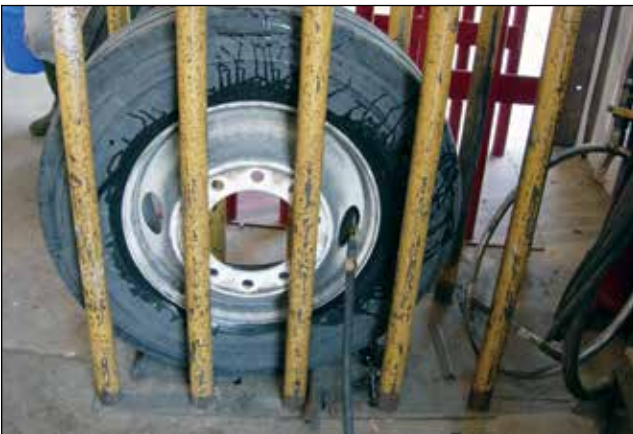
11 Place the assembly in the safety cage for safe inflation.
