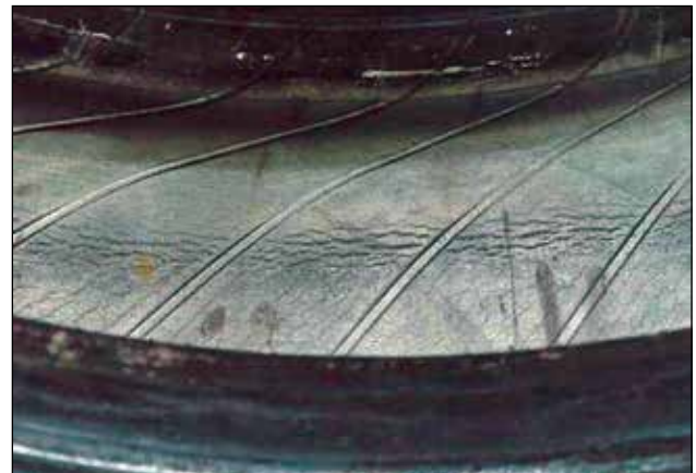
Sign of Run Flat Damage – Interior
