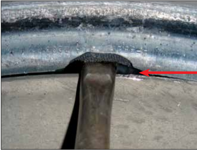
EFFECT: Bead Area or Inner Liner Damage CAUSE: Improper Demounting Procedure, Lack of Lubricant
