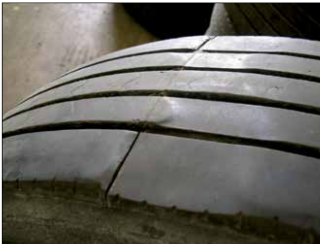
Open Splice Joint
