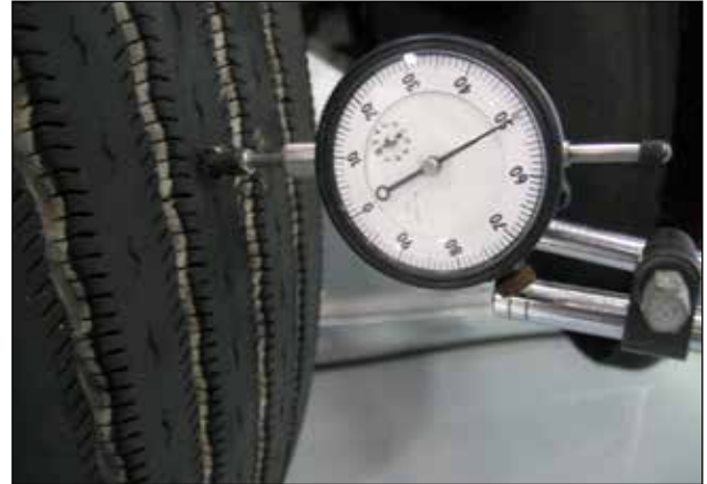
Measuring Radial Runout on Center Rib
