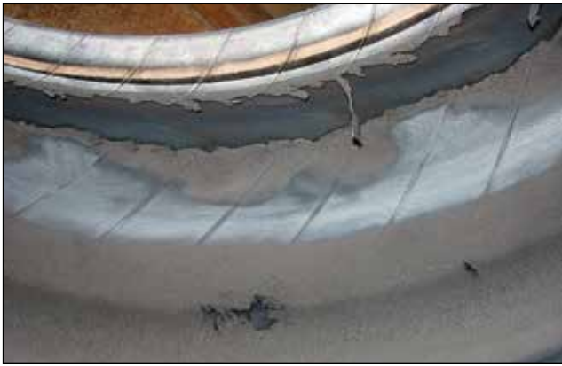
EFFECT: Discoloration, Blistering, and/or Separations of the Inner Liner CAUSE: Continued Operation After Loss of Tire Pressure
