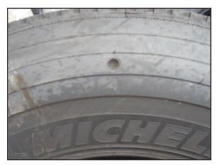
Prior to rotating the tire sidewall, the sidewall should be examined to make sure there are no cords exposed or cuts deeper than 3 mm. If these conditions exist, the tire should be removed and scrapped.
